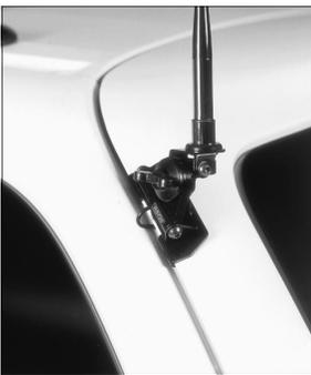
**Universal Lip Mounts:** Our universal lip mounts can be used on trunk lids or attached to almost any lip on a vehicle: Vertical, horizontal or anywhere in between. They are designed to fit over an edge no more than 1/4" thick, so check the thickness of the lip you want to mount to before you decide on the location. The mounts adjust in several planes so the antenna can be made vertical from virtually any angle.
