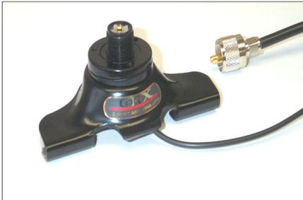
**Trunk lip mounts:** Our trunk lip mounts come with coax and are designed only for trunk lip use. They are adjustable to compensate for the angle of the trunk, but only up to 17 degrees. They are designed in Japan to fit on even the tightest tolerance gap between the trunk and fender.
