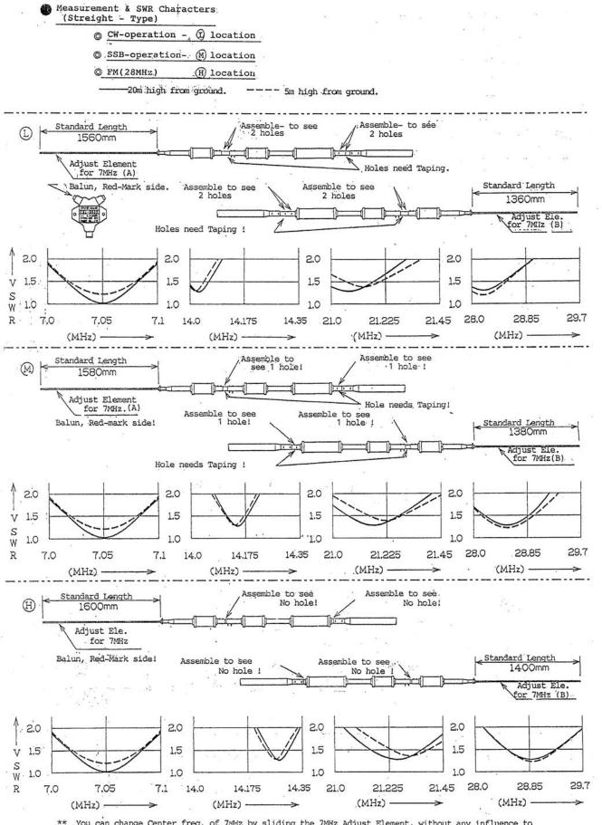
You can change Center freq. of 7MHz by sliding the 7MHz Adjust Element, without any influence to other frequencies. Shift of 7MHz band per each 1cm, is 15KHz.
