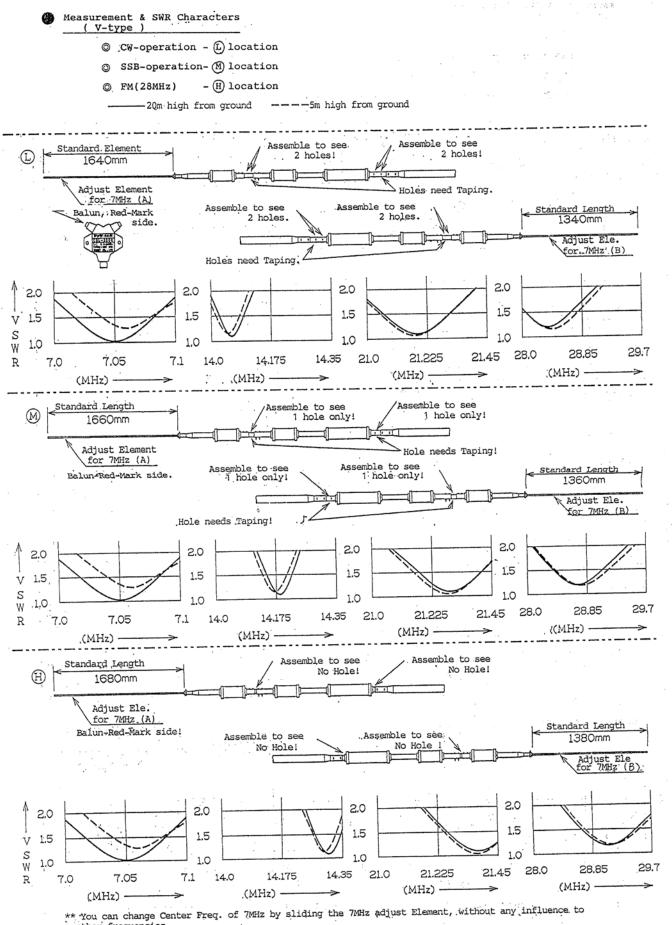
other frequencies. \*\* Shift of 7MHz band per each 1cm, is 15KHz. \*\* Difference of Left & Right 7MHz Element is to be 300mm.
